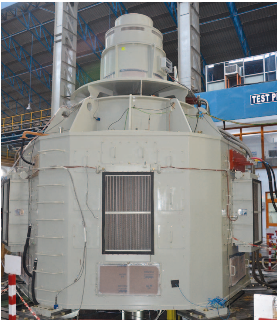
▼ Generator of HPP Kal during testing
