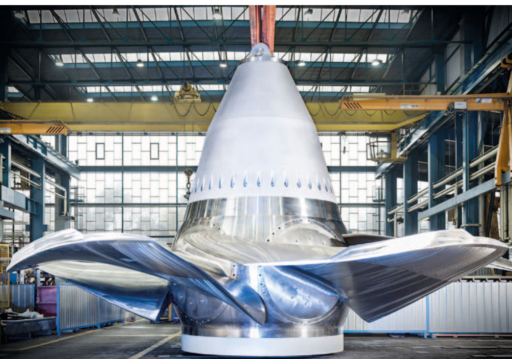
▼ Kaplan runner in the ANDRITZ HYDRO manufacturing workshop
