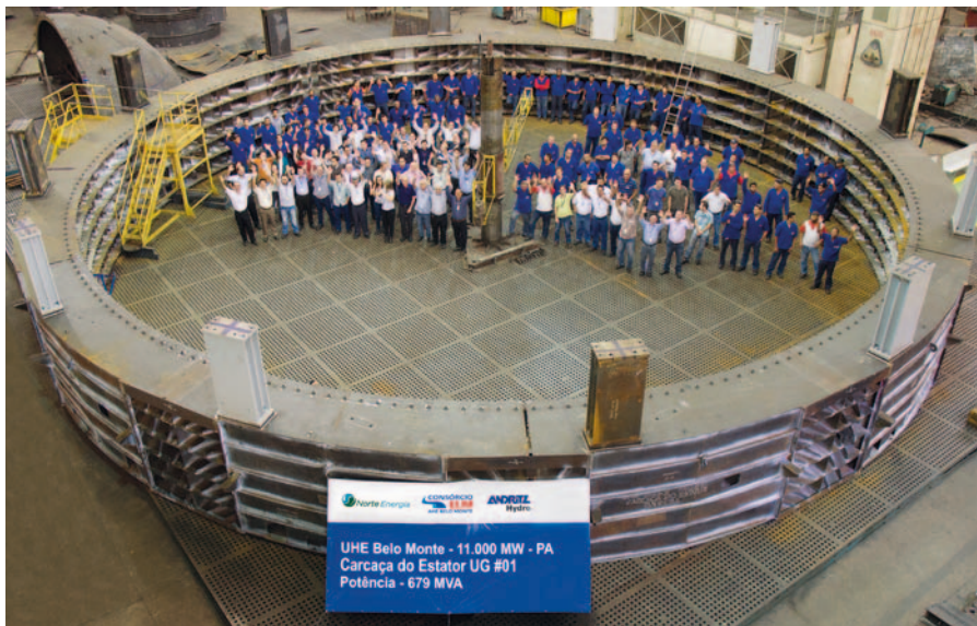
▼ Stator for HPP Belo Monte during manufacturing
