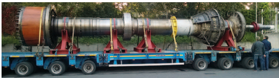
▲ Transportation of the line shaft (length: 14.8 m, weight: 95 tons)
