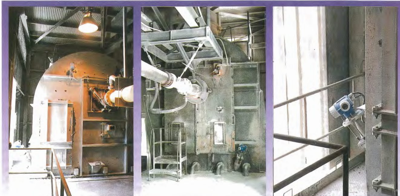
Kiln No. 1 (left), kiln No. 2 (centre) and the microwave sensor, which is mounted to the side of the firing hood (right).
