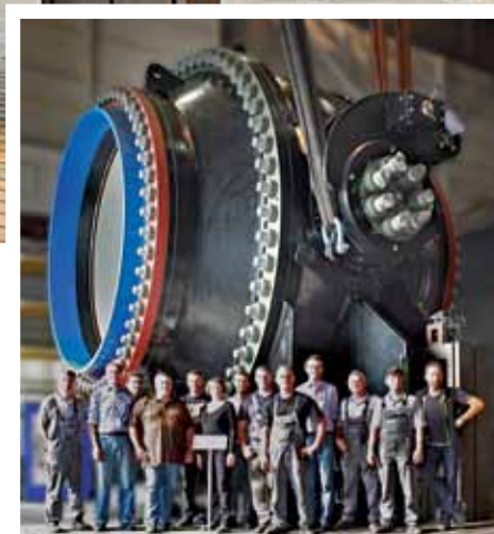
▲ Spherical valve for HPP Herdecke: completion of tightness testing after service
