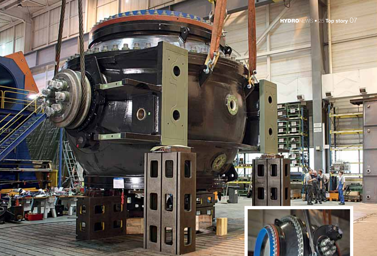
▲ Spherical valve for HPP Herdecke during assembly in the workshop
