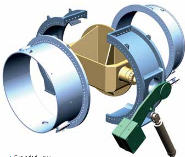
▲ Exploded view: main components of butterfly valve
