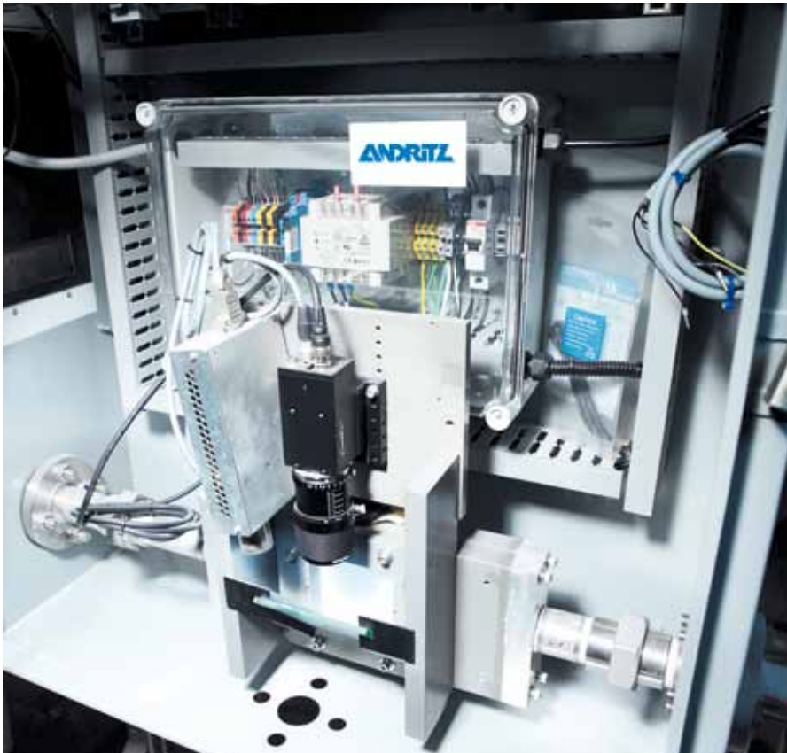
▲ Like a movie camera, the camera inside PulpVision® takes 24 pictures a second with a resolution from 7 to 100 microns. Dirt particles in the pulp are counted and computer-analyzed for size and size distribution.
